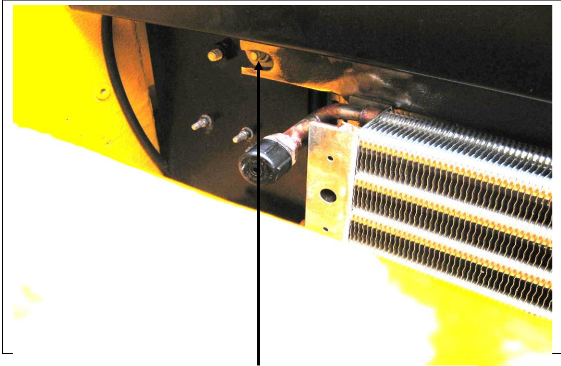
Top left mount bolt. Remove nut and washer, install bracket, and replace nut and washer.
